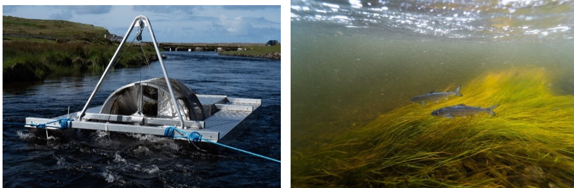
Images: Screw trap in operation at Butler's Pool (left) Salmon smolts released from screw trap at Butler's Pool (right)
