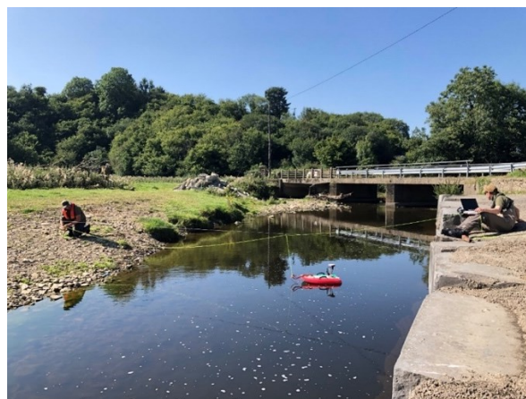
Image: Measuring flowing using an acoustic doppler current profiler (ADCP) on the Dinin River, Co. Kilkenny
