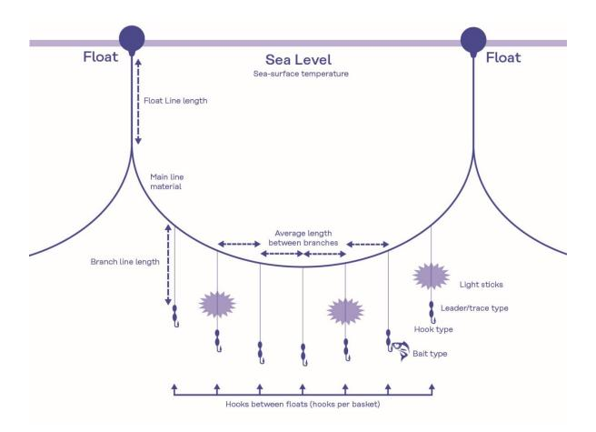
Longline (Gear Configuration): Average branch line length (meters): straight length in meters between snap and hook. Translation: Float Sea level Sea-surface temperature Float line length Main line material Average length between branches Branch line length Light sticks Leader/trace type Hook type Bait type Hooks between floats (hooks per basket)
